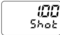
Example) 6-digit type One-shot output time setting mode displayed (Example shows default value displayed)
